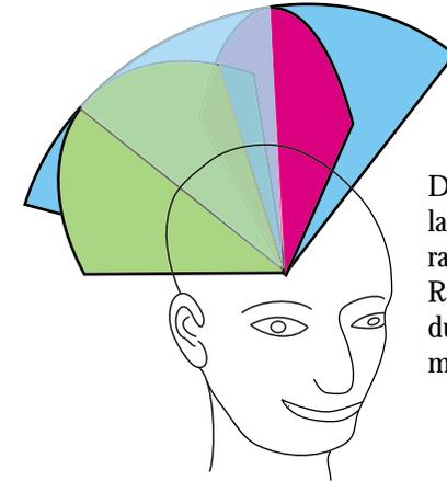
Diagram of arcs of overlapping pencil beams of radiation in Stereotactic Radiosurgery to produce small area of treatment in the brain
